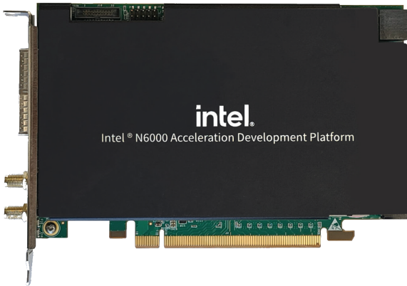
Figure 10. Physical view of the Intel FPGA SmartNIC N6000-PL Platform board.
