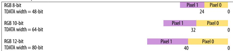
**Figure 29. TDATA RGB Layout: Four pixels in parallel configuration**
