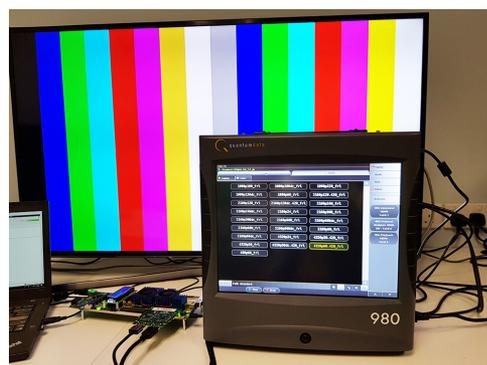
Figure 3. Intel's HDMI 2.1 IP passing QD980 protocol tester 8K data rate
