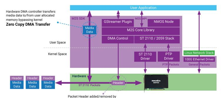
ST 2110 IP FPGA HW Engine
